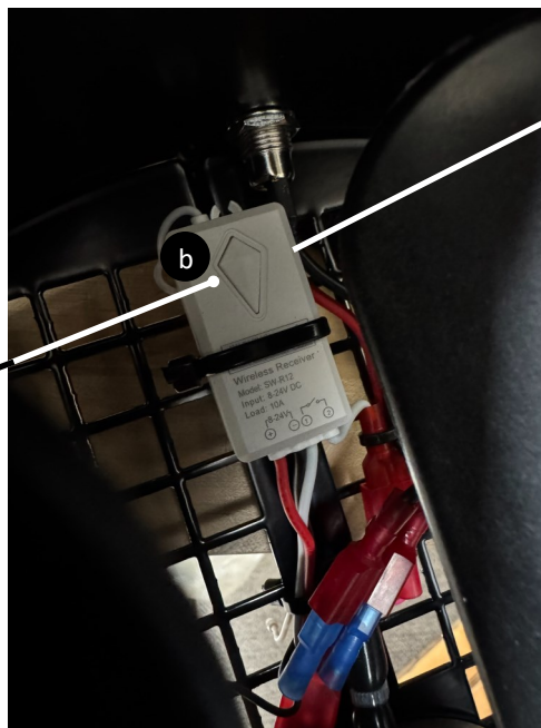
Press receiver button and hold for 3 seconds until red light begins flashing.
